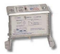
WD1-DS models include fail-safe circuitry to signal an alarm condition for an internal malfunction or loss of power to the sensor. The WD1-DS models incorporate a reverse acting set of relay contacts that are closed in a normal condition.
